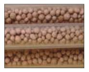
Bio-ceramic granulate contained in the AIFIR filter is the product, which is made of various kind of ceramics, mixed with mineral oxides like Silica Oxide (SiO2), Aluminum Oxide (Al2O2), etc. The mixture of these materials will emit FIR (far-infrared rays)
