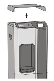
3.Use screwdriver to remove the screws on the top cover, left and right plate. After removing top cover, get off the insulator board, press cold-water and hot-water taps, completely drain out all water. It is ready for clean.
